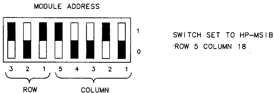
Figure 2-2. Module Address Switch
