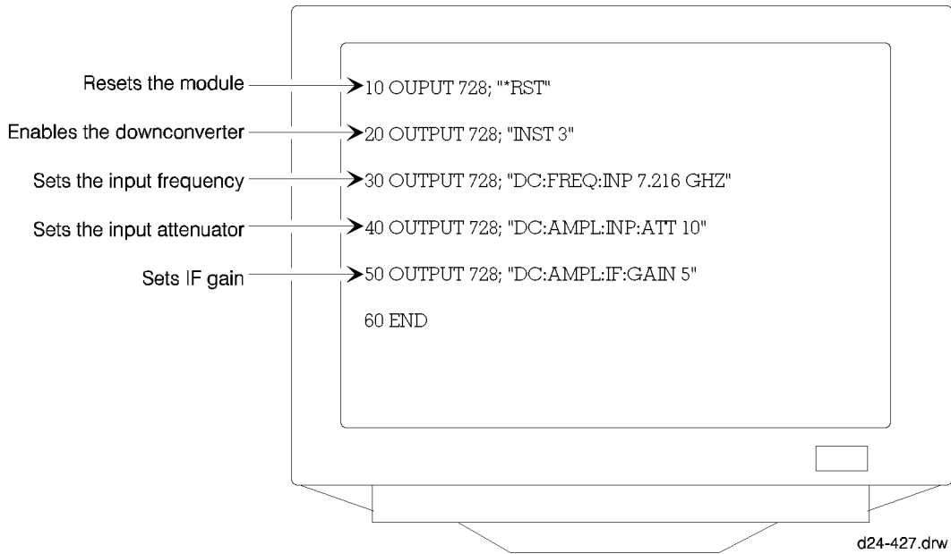
Figure 2-26 HP BASIC on an HP 9000 series 200/300 Controller
