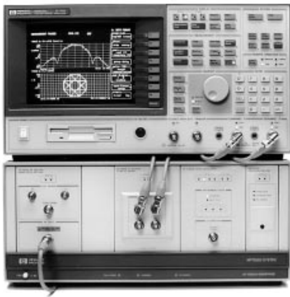
Figure 1. HP 89410A vector signal analyzer and HP 71910A wideband surveillance receiver together form a wideband vector signal analyzer system.
